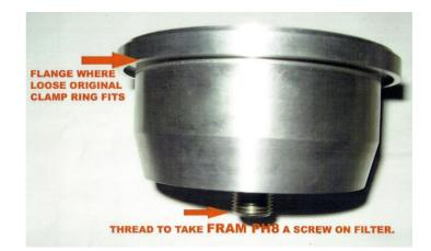
Fitting the adaptor is straightforward but it will be necessary to check the clearance between the two seals:
